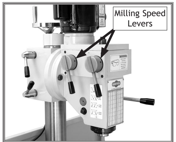
Figure 52. Gearbox and controls.
